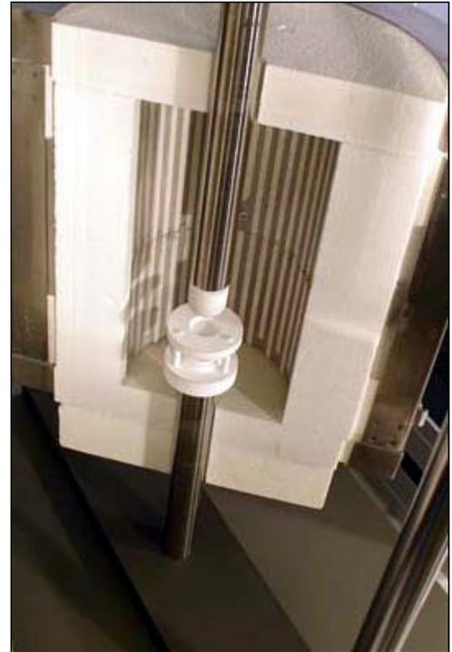
*ASTM C1499 defines equibiaxial flexural strength as the maximum stress a material is capable of sustaining when subjected to flexure between two concentric rings. Flexure cupping of a circular plate is caused by loading an inner load ring and outer support ring. Equibiaxial flexural strength is calculated from the maximum-load of a biaxial test carried to rupture, original dimensions of the specimen, and Poisson's ratio.*
