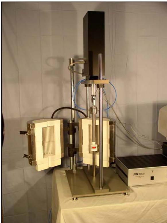
Researchers at The Ohio State University use a TestResources dual column 100R PC Controlled test system to perform tests at low forces. The modular actuator includes a position encoder (0.007 micron resolution) that enables slow constant rate of loading and position control. The system includes furnace and high temperature extensometry for strain control.
