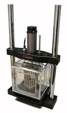
Vascular devices are tested for fatigue life up to 400 million cycles. 800L system shown is designed for high speed high frequency tests in a saline bath with 15 test samples all tested simultaneously.
