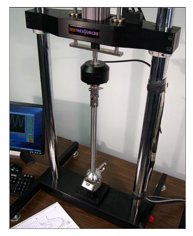
Orthopedic devices implanted in the body must undergo static and fatigue tests that mimic ten years of product life to be considered acceptable. Spinal implants and constructs are tested according to various ASTM and ISO standards and typically require static tension, compression and torsion testing, and fatigue tests. The typical medical device developer needs a versatile proven test system that can do both types of tests and one that can expand to combined axial torsional loading.
