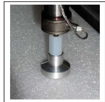
800LE3 - rated 6 kN with a lower force 1000 gf full scale load cell. The encoder measured position.
