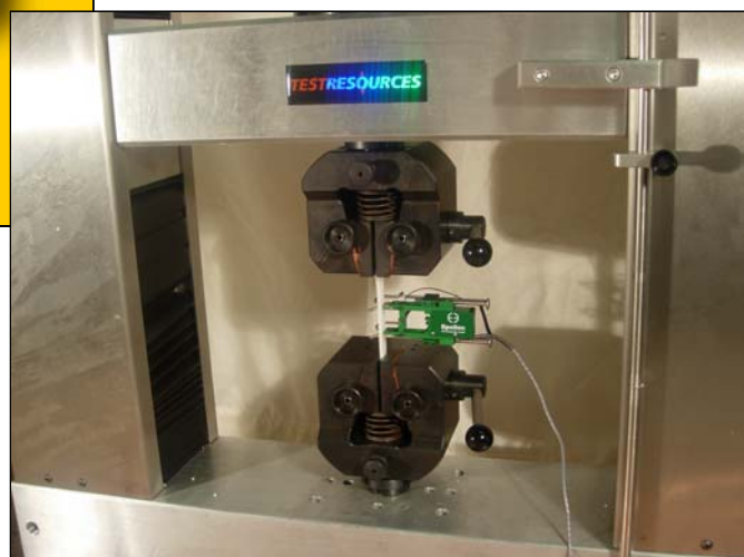
11KM with Wedge Action Grips & Extensometer performing tensile test on composite test sample.
