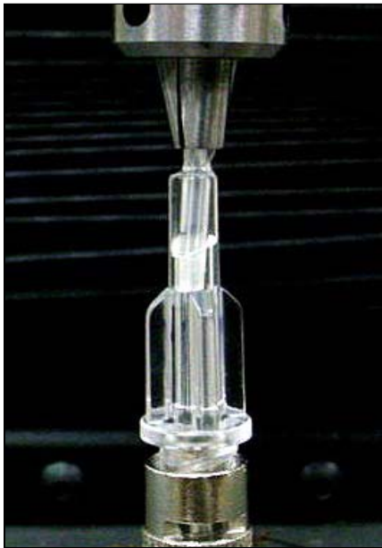
TestResources 200R Test System with Collet Grips perform Catheter Luer Fitting Tensile Strength Test
