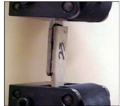
TestResources G7-1 Roller Capstan Grips used for lap shear tests on plastics.
