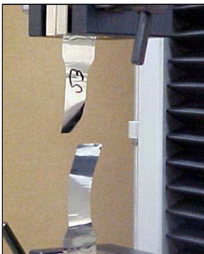
TestResources G240K Vise action grips performing strength tests on stainless steel foil.
