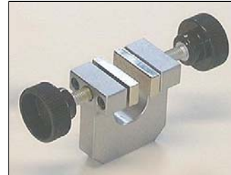
G227SS Stainless Steel Vise Grip * Rated 440 N (100 lb) * Tare weight ~240 g with jaws * For specimens to 6 mm thick * Female 10-32 UNF (M5) thread * Fatigue or static
