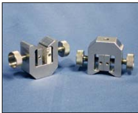
G140SS Stainless Steel Vise Grip * Rated 200 N (50 lb) * Tare weight ~120 g with jaws * For specimens to 8 mm thick * Jaws 15 X 15 mm (0.6" X 0.6") * 10-32 F (M5) thread
